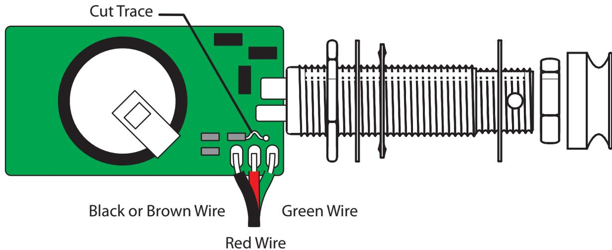
1. Position the Simple Jack circuit board so that the round super capacitor is facing upward and the 1/4" output jack is to the right.
